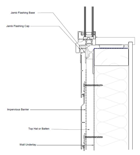
Horizontal Cladding - Sill Detail
