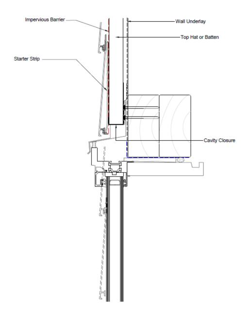
**Horizontal Cladding - Window Head Detail**
