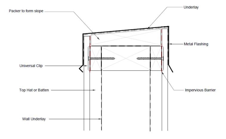
Vertical Cladding - Parapet Flashing
