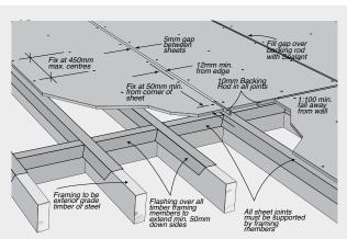
Note: 15mm - maximum span 450mm centres. 18mm - maximum span 600 centres.
