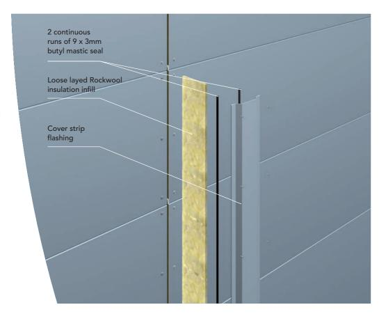
18. Continue to install panels around the building in accordance with our standard details. Full key details are available on request.
