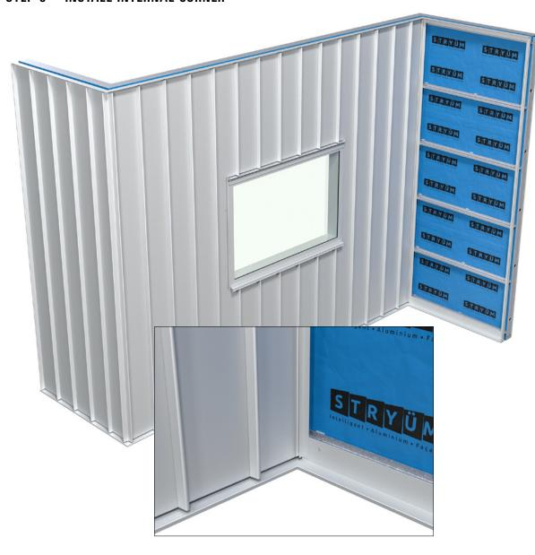
Install TRM0201b Female into the internal corner.
