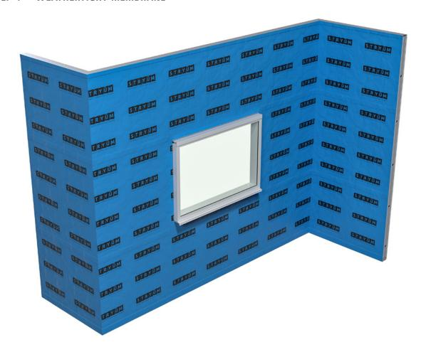
As Stryüm is a rainscreen façade, a weathertight membrane must be installed over the supporting wall. This membrane needs to meet the project specific requirements for weathertightness and be installed as per manufacturers guidelines. All penetrations through the membrane must be sealed.
