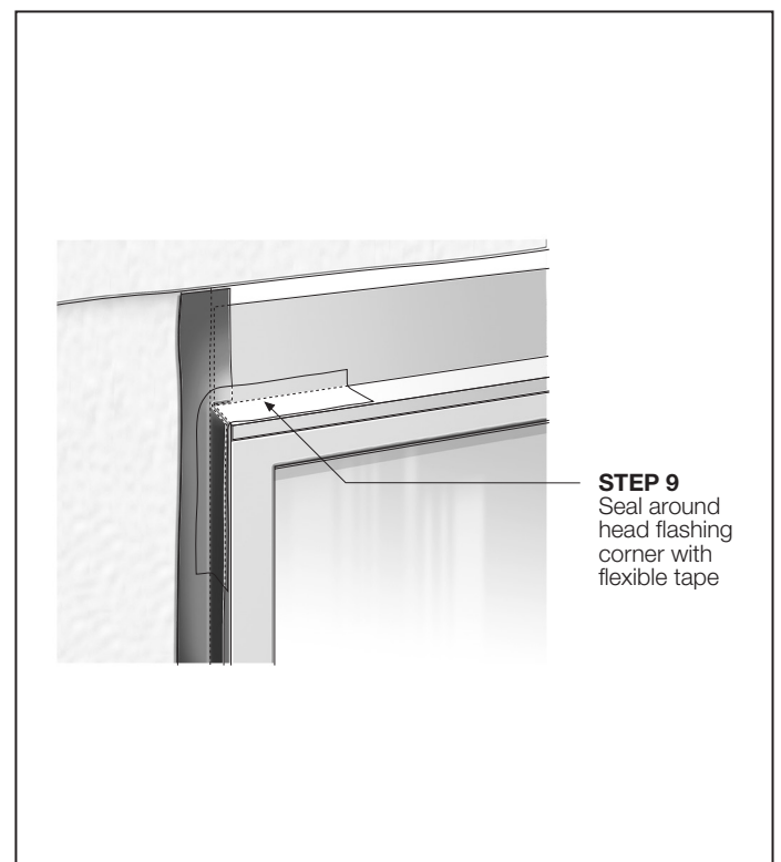
FIGURE 38 INSTALLATION OF WINDOW
